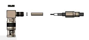
2) Open the cable braid and slide the tube over the dielectric and under the braid. Insert the centre core into the insulator then slide the cable into the body, ensuring that the cable braid is on the outside of the connector mandril and that the centre core locates in the internal mounting post.
