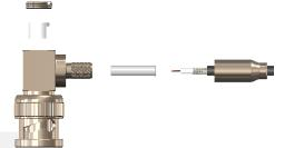
2) Open the cable braid and slide the insulator tube over the dielectric and under the braid. Insert the cable into the body, ensuring that the cable braid is on the outside of the connector mandril and that the centre core locates in the internal mounting post
